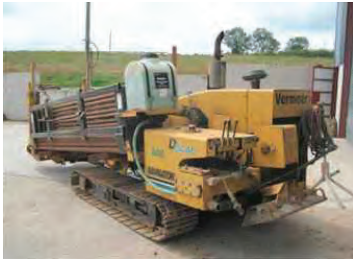
Typical Directional Drilling Rig
